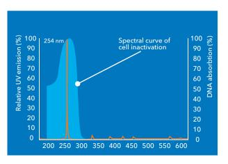
The monochromatic ECORAY UV lamp emits at a wavelength of 254 nm, which is in the maximum of the effective disinfection range of the spectrum
