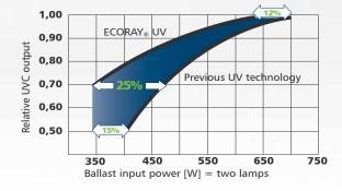
Ecoray UV lamps are more efficient, longer-lasting, more stable and more sustainable than previous Wedeco UV lamp technology. For minimized power consumption the lamps can be operated in dim mode, delivering the exact UV output required to meet the needs of various operating conditions.
